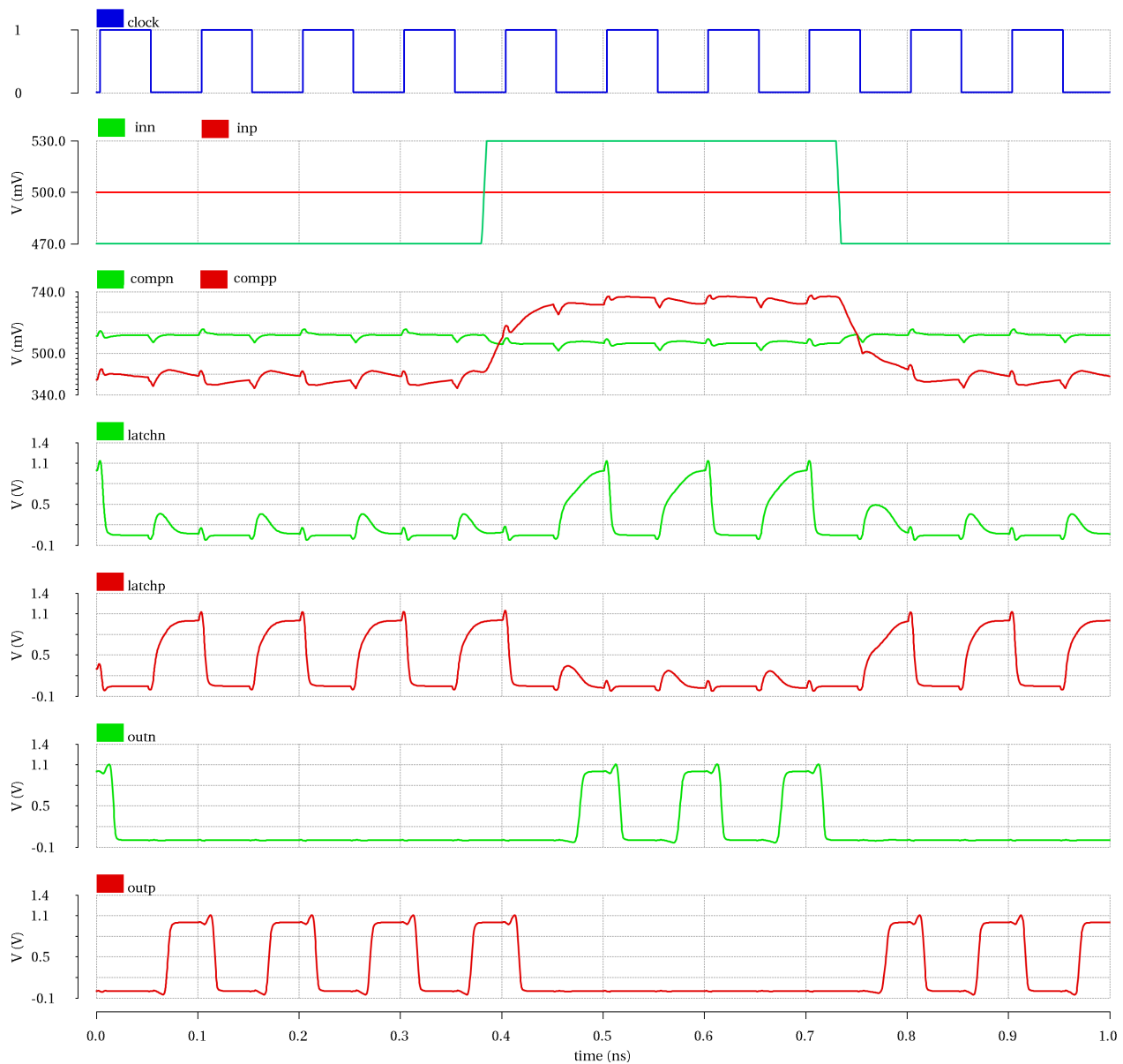
Figure 3. The results of transient simulation of the base (uncompensated) design.
