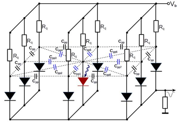
Fig. 4. A simplified equivalent circuit of the MPPC S12572-010 with high pixel density.
