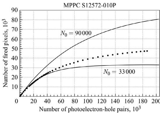
Fig. 2. The response of the MPPC S12572-010P with a total number of pixels  $N_0 = 90\,000$  exposed to light from a laser with a pulse width of 40 ps. For comparison, theoretical functions (1) with  $N_0 = 90\,000$  and  $N_0 = 33\,000$  are shown.
