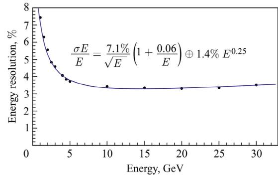
Fig. 5. The dependence of the energy resolution of the ECAL0  $3 \times 3$  module matrix read out by the MPPC S12572-010P on the electron beam energy.
