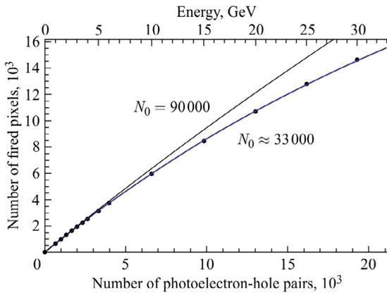
Fig. 1. The dependence of the response of the ECAL0 cell read out by the MPPC S12572-010P on the electron beam energy, and the average number of the photoelectron-hole pairs produced in the MPPC.
