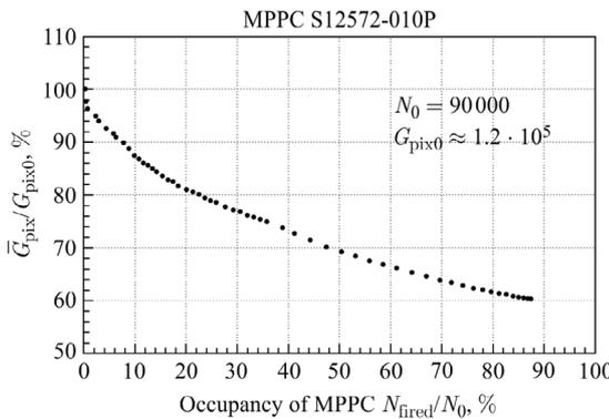
Fig. 3. The dependence of the average MPPC S12572-010P gain on the occupancy of pixels.
