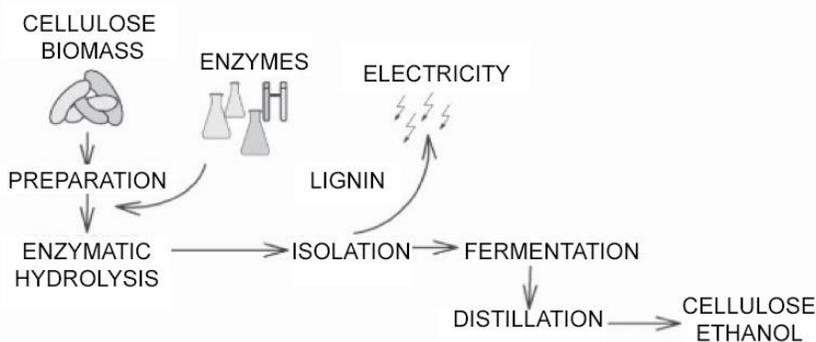
Fig. 1. Ethyl alcohol production process by Iogen Corporation [6]
