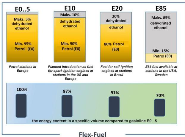
Fig. 3. Example ethanol fuels together with a comparison of energy content [8]
