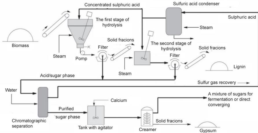
Fig. 2. Ethanol production process by BlueFire Ethanol Inc. based on sulphur acid for hydrolysis of plant biomass [6].
