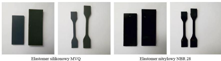
Fig. 4. Impact of bioethanol fuel on elastomers [9]
