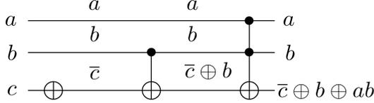
Figure 2. A reversible circuit with a NOT, CNOT, and Toffoli gate.
