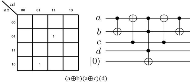
Figure 8. Karnaugh map and POE reversible circuit realization for function  $F_2 = ab'cd \oplus a'bcd$ .
