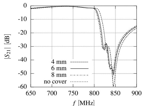
Fig. 8. Transmittance of filter FZ835 tuned by changing the height of cover's mounting – measured data.
