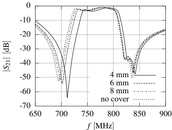
**Fig. 10.** Transmittance of filter FPP794 tuned by changing the height of cover's mounting – measured data.
