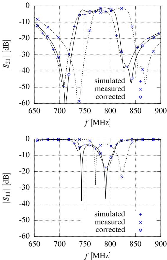
**Fig. 9.** Transmittance and reflectance of filter FPP794 for blocking signals in the ranges 825 MHz to 845 MHz and 690 MHz to 730 MHz.
