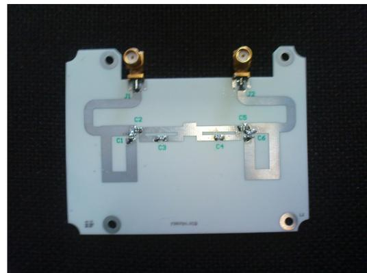
Fig. 4. Printed circuit board of filter FPP794.
