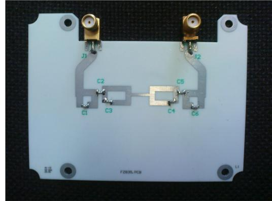
Fig. 2. Printed circuit board of filter FZ835.
