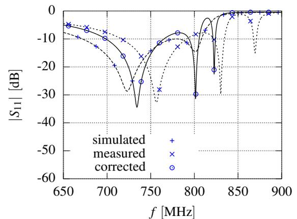
Fig. 7. Transmittance and reflectance of filter FZ835 for blocking signals occupying bandwidth 825 MHz to 845 MHz.
